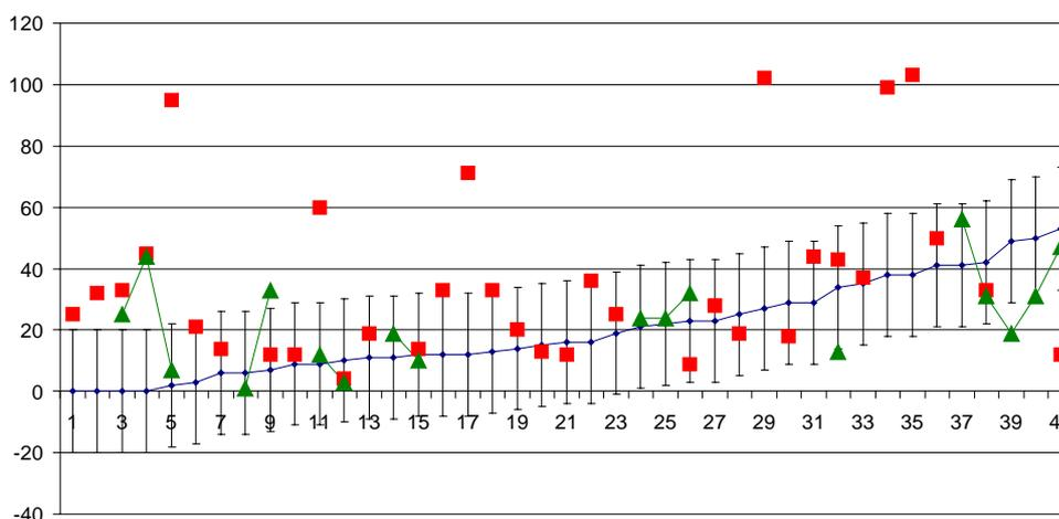
Nearly 80% of the precise levels (▲) fall within +/- 20% of the modelled profile (■). The soils (■) show a wide dispersion, with very little fit. We can see from the data that the model tends to under-predict low order movement (less than 20mm) but is more accurate than the soils test over the remainder of the range, and consistently so.
