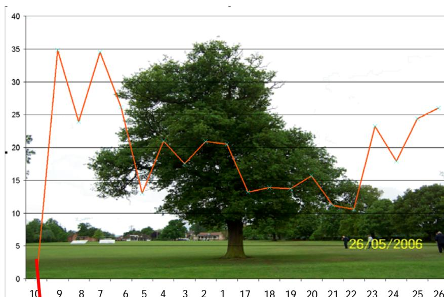
The datum, sunk to a depth of 10mtrs in sandy gravel, is to the extreme left - Station 10. We can see that Stations 7 & 9 have moved 35mm in total. Stations 21 and 22 have moved least - just over 10mm.
