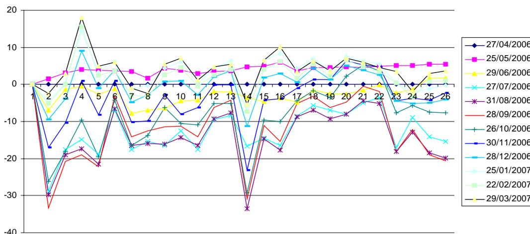
This provides some idea of the magnitude of movement between dates and differences between the wettest (top line in both cases) and driest times (lowest line) of the year, showing which stations move most. It's an indicator of clay activity and mineralogy across the site as well as rainwater penetration.
