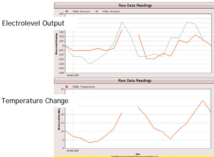
Electrolevels have measured movement in the range of -0.04 to 0.05 = 0.09 degrees. The temperature change in that time has been 22 degrees.
