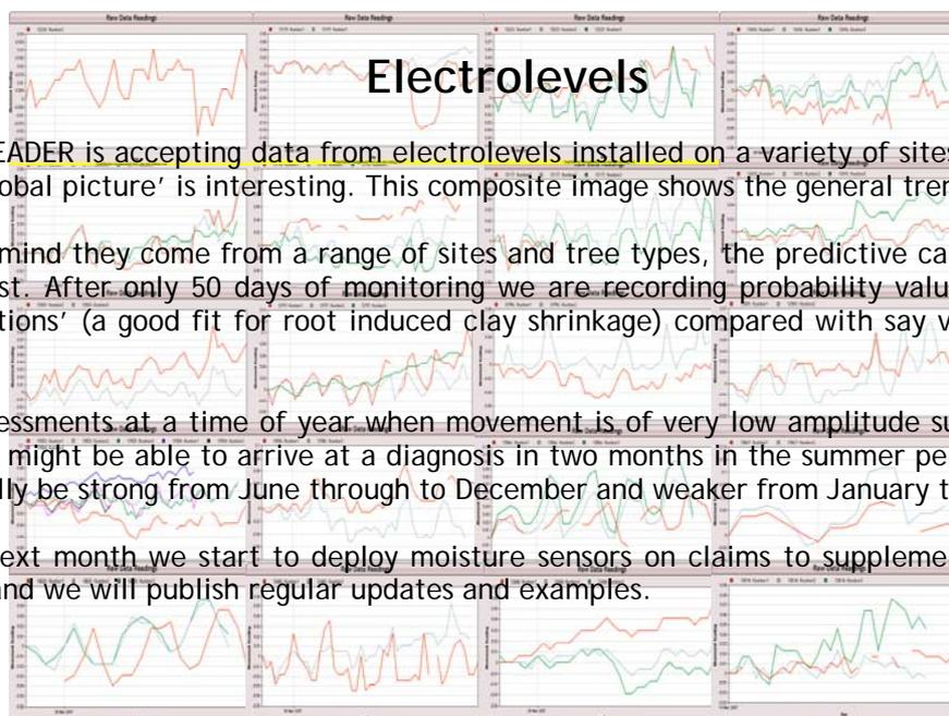
The DataREADER is accepting data from electrolevels installed on a variety of sites across the UK, and the 'global picture' is interesting. This composite image shows the general trendlines.
